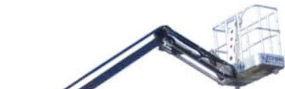
The large fly-jib is designed for maximum travel and flexibility.
