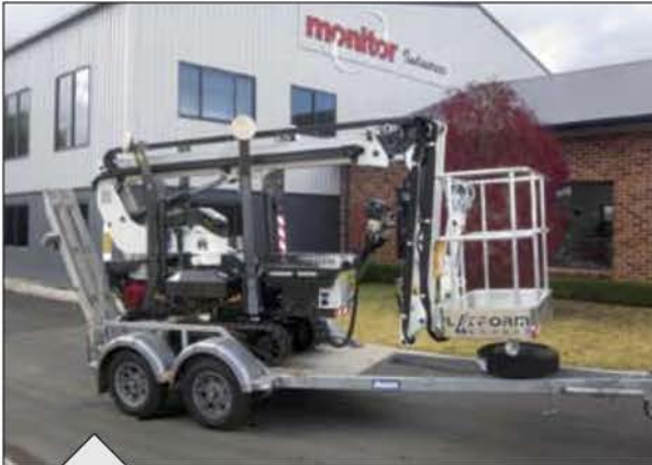
Extremely light weight and compact stowed size allows easy transportation. This package including the steel trailer weighs under 2t.
