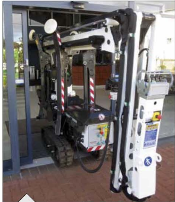
The light-weight basket is simple to remove in less than one minute, allowing very narrow access and a stowed length of only 3.69m
