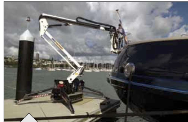
Weighing under 2 tonnes, the 1575 is ideal for use on load sensitive floors, including jetties!
